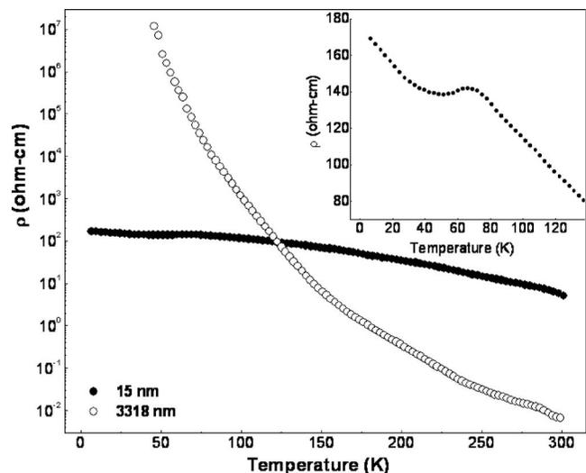
FIG. 6. (Color online) Resistivity vs temperature curves for PCMO pellets with two different particle sizes. Inset shows the resistivity vs temperature curve for the nanoparticle sample in the low temperature region.
