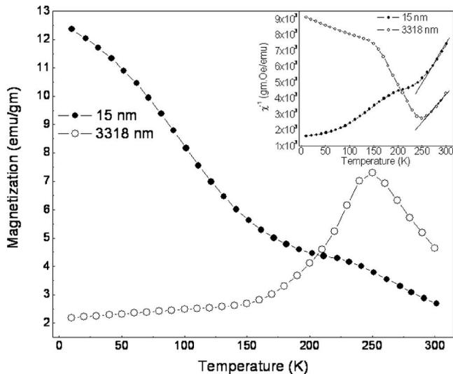
FIG. 4. (Color online) Magnetization vs temperature for bulk and nano-PCMO under a magnetizing field of 2 T.
