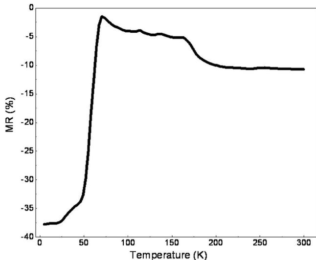
FIG. 8. (Color online) Negative MR curve for PCMO pellet (particle size  $\sim 15$  nm).
