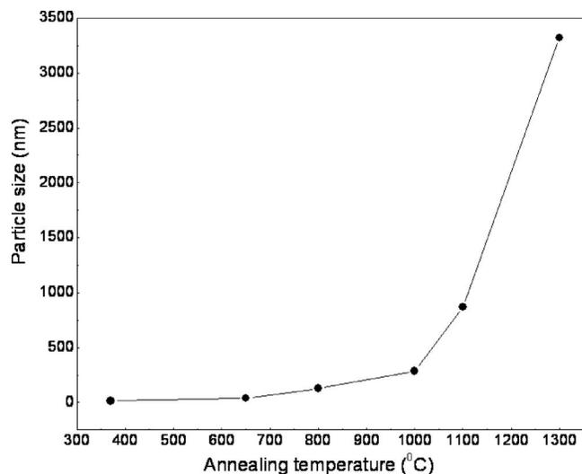
FIG. 2. (Color online) Variation of average particle size with the annealing temperature.
