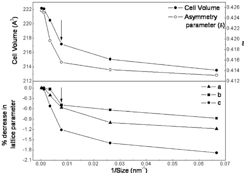
FIG. 3. (Color online) Variation of cell volume, asymmetry parameter, and change of cell parameter with particle size.
