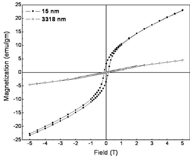
FIG. 5. (Color online) Magnetization vs magnetic field for bulk and nano-PCMO at a temperature of 5 K.
