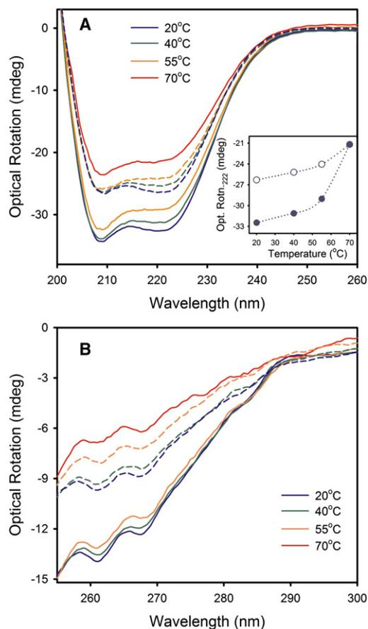
FIGURE 1 Far-UV (A) and near-UV (B) circular dichroism (CD) spectra of HSA in aqueous PBS buffer at different temperatures. (Solid lines) Thermal unfolding (forward, heating) process. (Dashed lines) Refolding (reverse, cooling) process. (A, inset) The change in the optical rotation at 222 nm for both heating (solid symbols) and cooling (open symbols) processes. (Dotted lines) Guide to the eyes.
