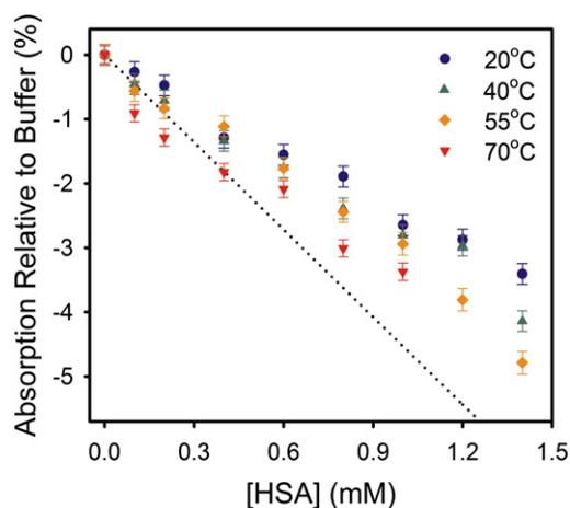
FIGURE 2 Concentration-dependent THz absorption relative to buffer of HSA in PBS buffer at four different temperatures measured with a p-Ge THz spectrometer in the range of 2.1–2.8 THz. (Dotted line) Two-component water displacement model.
