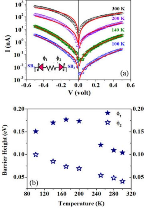
Fig. 8. (a)  $I$ - $V$  data with fitted to (1) at few representative temperatures. (b) Variation of barrier heights  $\phi_1$  and  $\phi_2$  with temperature.
