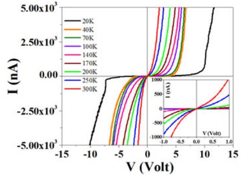
Fig. 4. Nonlinear  $I$ - $V$  characteristics of the Si NW MSM device at different temperatures. Inset shows the data at low bias voltages  $\approx \pm 1 \text{ V}$ .
