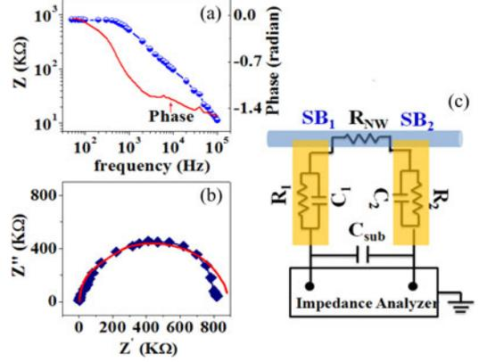
Fig. 6. (a) Plot of total impedance  $Z$  and the phase with frequency at 300 K. (b) Nyquist plot  $Z'$  versus  $Z''$  for the whole device. (c) Equivalent  $R$ - $C$  network for the Si NW device.
