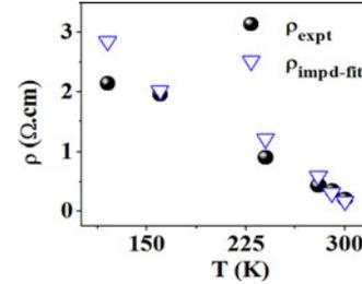
Fig. 7. Comparison of two  $\rho$  values obtained from direct dc resistivity measurement and from the  $R$ - $C$  model fit of impedance spectroscopy.
