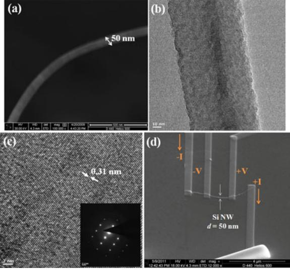
Fig. 2. SEM image of (a) single NW before device fabrication, (b) TEM image of a Si NW, (c) HRTEM image showing lattice fringes. The inset shows SAED pattern, and (d) Single Si NW device with four Pt-electrodes fabricated by e-beam-assisted deposition.
