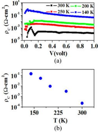
Fig. 5. (a) Bias dependence of specific contact resistance  $\rho_C$  at few representative temperatures. (b) Temperature dependence of  $\rho_C$  at bias 0.4 V.
