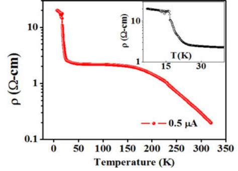
Fig. 3.  $\rho$  versus  $T$  plot with current bias  $0.5 \mu\text{A}$ . Inset shows that  $\rho$  increases sharply below  $30 \text{ K}$ .
