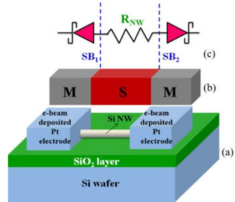
Fig. 1. (a) Schematic diagram of a Si NW with e-beam deposited Pt contact electrodes. (b) Representative MSM structure of the NW device with an equivalent circuit constituted by two Schottky diodes connected back to back with a series resistance  $R_{NW}$ .
