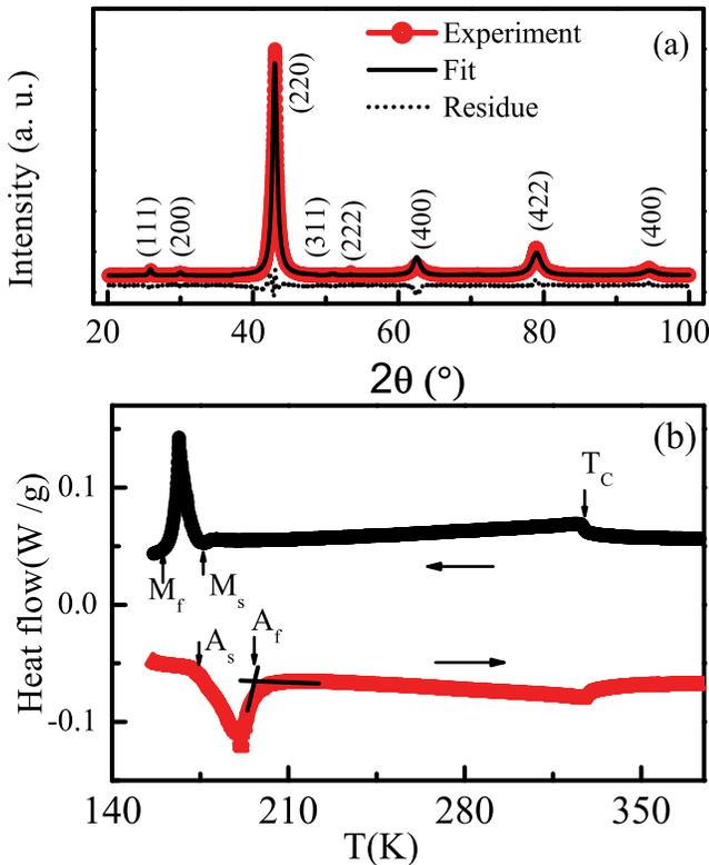
FIG. 1. (a) Room temperature XRD pattern along with the fitted pattern and residue. (b) DSC curve as function of temperature. One of the straight line intersections are shown, which was used to determine the transition temperatures.
