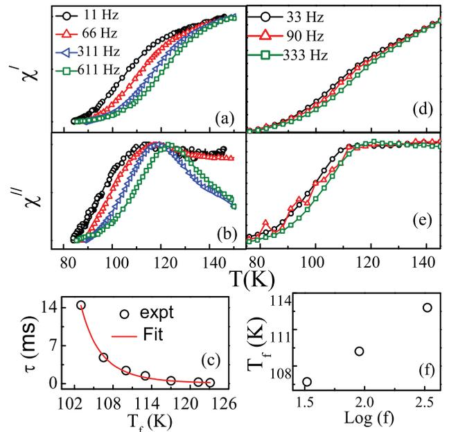
FIG. 4. Normalized frequency dependent (a) real ( $\chi'$ ) and (b) imaginary ( $\chi''$ ) of a.c. susceptibility as a function of temperature in zero d.c. field. Figure (c) shows experimental data fitted with dynamical scaling law for phase transition. Figs. (d) and (e) show  $\chi'$  and  $\chi''$  at 700 Oe d.c. field and Figure (f) shows shift of  $T_f$  with frequency at d.c. field of 700 Oe.
