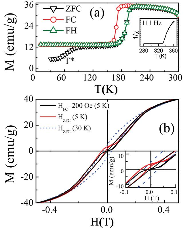
FIG. 2. (a) ZFC, FC, and FH at the field of 500 Oe as a function of temperature. The inset in 2 (a) shows inverse real χ' at 111 Hz. (b) Full MH curve measured after FC at 200 Oe and ZFC at different temperatures. The inset in Fig. 2(b) shows the expanded region near zero field.
