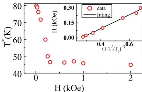
FIG. 3. H-T phase diagram,  $T^*$  is the freezing temperature at a given field. The inset shows fitting to Heisenberg model, up to 300 Oe as a function of reduced temperature.
