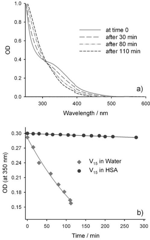
**Figure 1.** a) Absorption spectra of a very dilute solution of  $V_{15}$  in undegassed water at different time intervals. b) Time-dependent absorption profiles of  $V_{15}$  at 350 nm in water and HSA. From the kinetics an enhanced stability of  $V_{15}$ , especially against oxidation in HSA, is evident.
