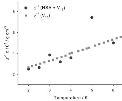
**Figure 2.** Inverse magnetic susceptibility  $\chi^{-1}=\alpha(\chi_{\text{total}}-\chi_{\text{HSA}})^{-1}$  of  $V_{15}$  in HSA with the diamagnetic contribution of the sample holder and HSA subtracted and a fitting parameter  $\alpha=1/5$ . The data are matched to the inverse susceptibility of bulk  $V_{15}$ . The experiments are performed in a magnetic field of 0.1 T.
