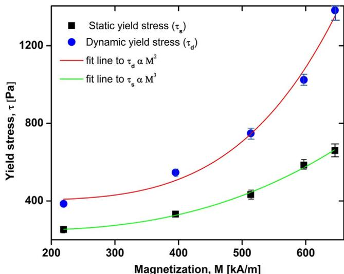
Fig. 4. Field-induced static (square) and dynamic (circle) yield stress for MR fluid as a function of particle magnetization  $M$ .
