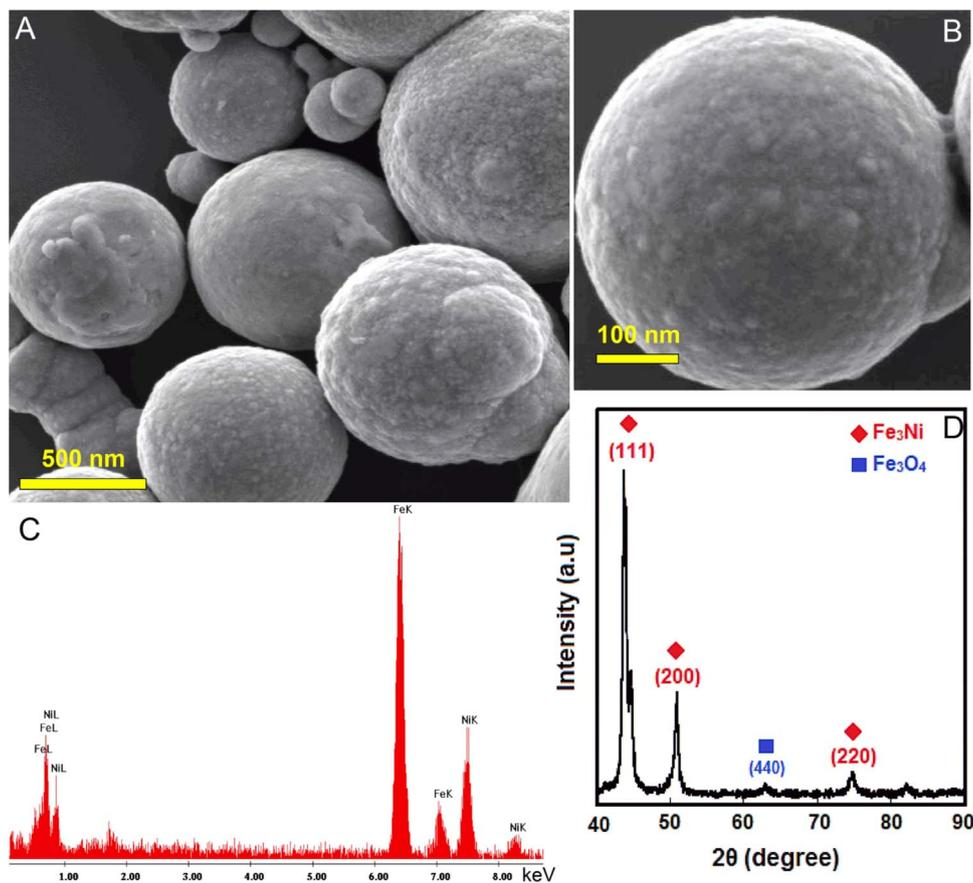
Fig. 1. (A, B) Low and high magnification FESEM images of PAA- $\text{Fe}_3\text{Ni}$ , (C) EDAX spectra and (D) X-ray diffraction patterns of  $\text{Fe}_3\text{Ni}$  microspheres.
