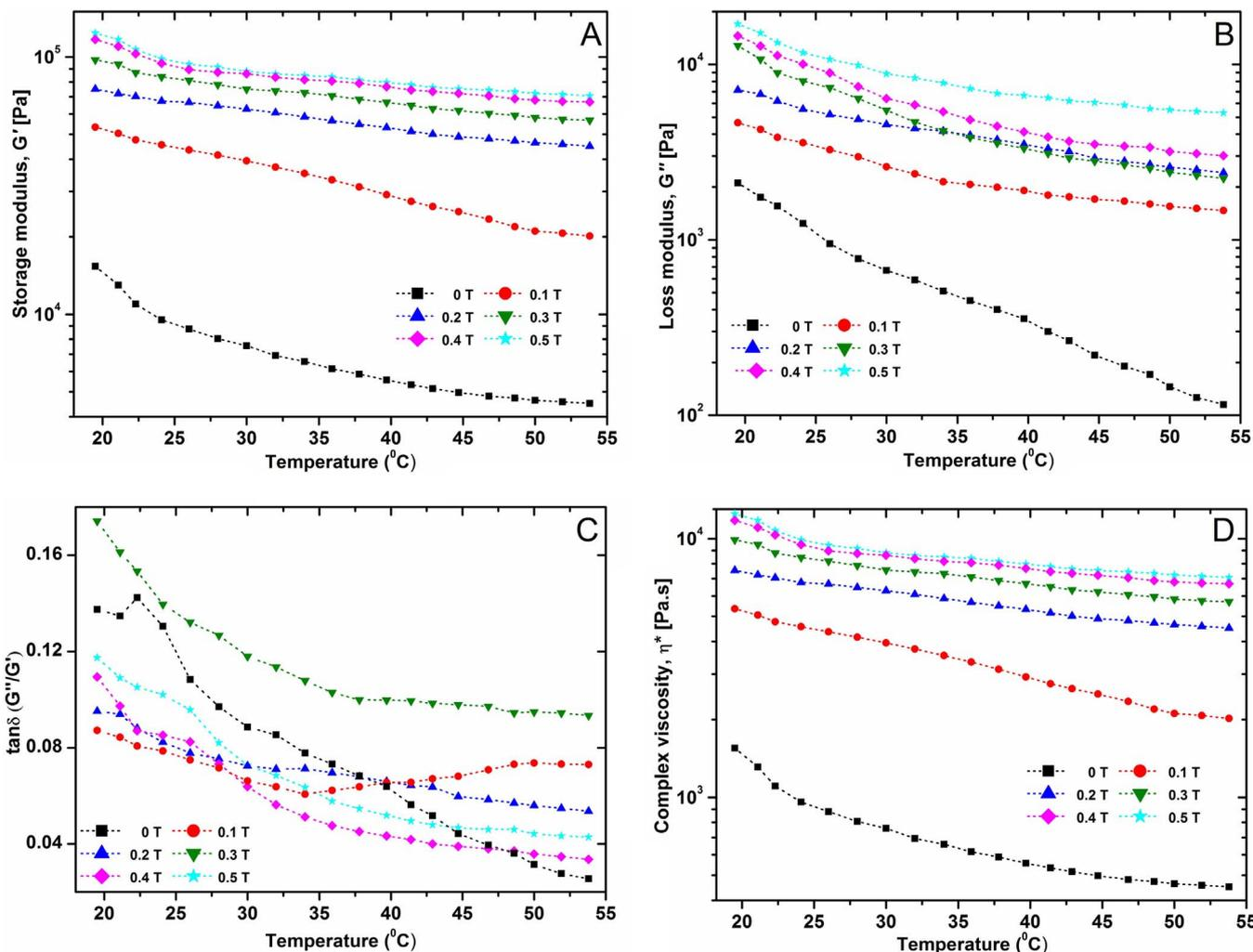
Fig. 5. Storage ( $G'$ ) and loss moduli ( $G''$ ) as a function of temperature and magnetic fields (A, B); loss factor versus temperature (C) and complex viscosity as a function of temperature (D) are shown.
