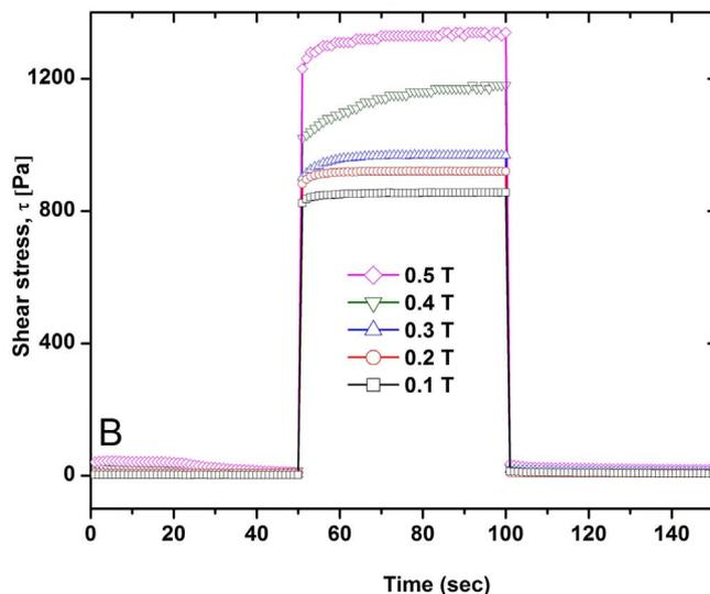
Fig. 3. (A) Steady shear rheological behavior of MR fluids for different magnetic fields. (B) Field-induced shear stress relaxation with time.
