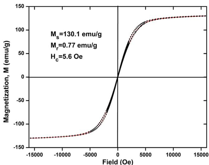
Fig. 2. Room temperature M-H hysteresis curve of PAA-Fe<sub>3</sub>Ni sample.
