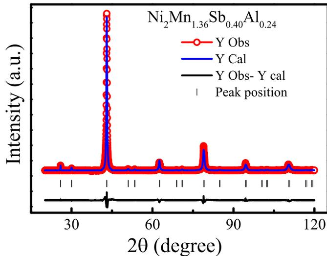
Fig. 1. XRD pattern obtained at 300 K along with calculated pattern, residue and peak position.
