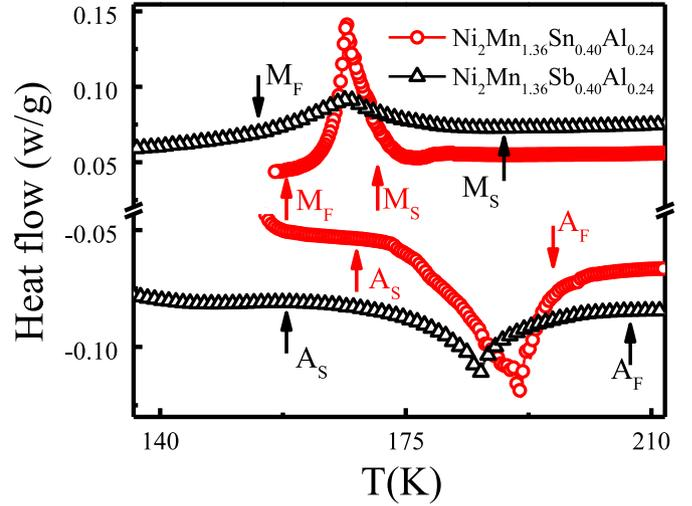
Fig. 2. DSC curves obtained for Sn and Sb based samples in cooling and heating cycle performed at the rate of 10 K/min.
