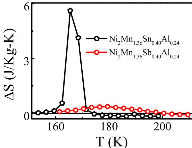
Fig. 4. Entropy change due to application of field of 1.5 T calculated from modified Maxwell relation.
