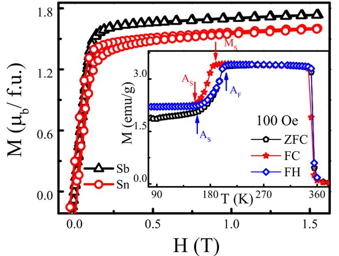
Fig. 3. Magnetic isotherms measured at 300 K for Sn and Sb samples in  $\mu_B/\text{f.u.}$ . Inset shows ZFC, FC, and FH at the field of 100 Oe as the function of temperature.
