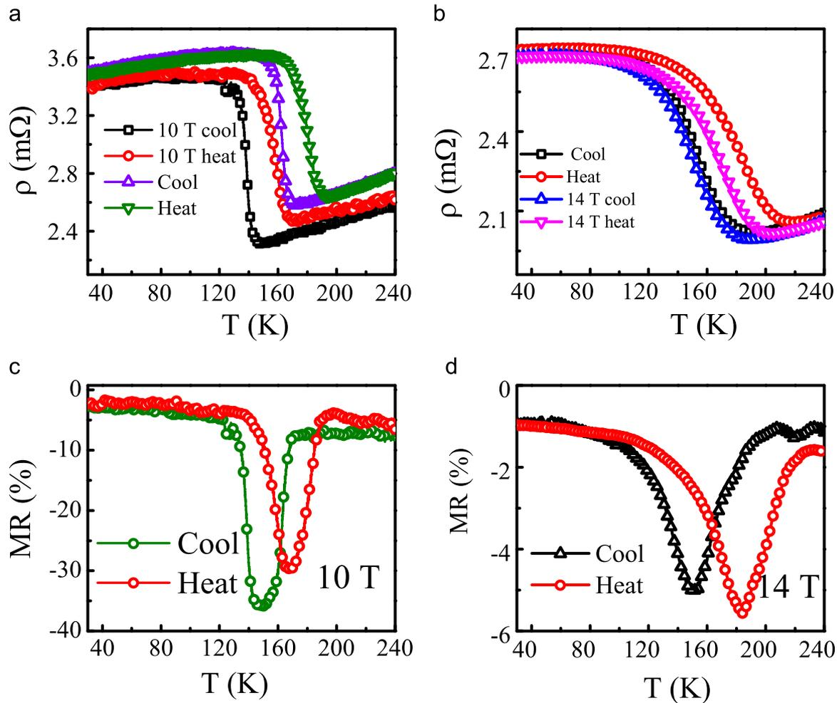
**Fig. 5.** (a) and (b) show resistivity measurement performed in the zero applied dc magnetic field and field of 10 T and 14 T for Sn and Sb alloy respectively. (c) and (d) show MR obtained for respective alloys.
