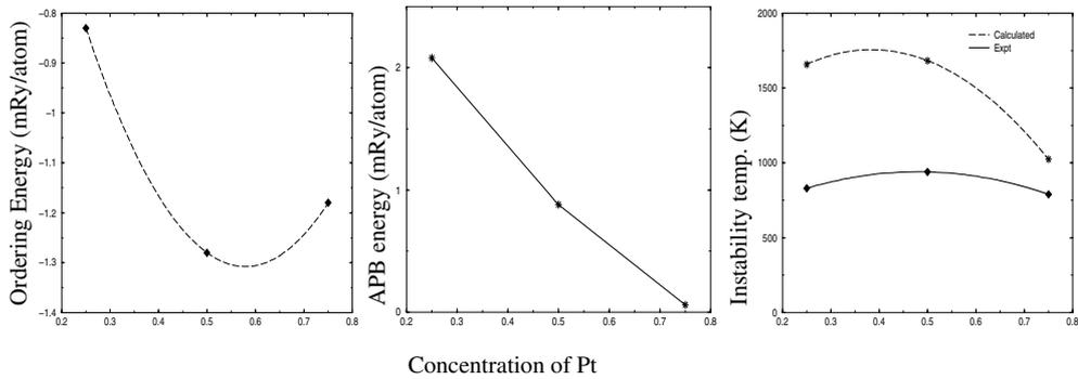
**Figure 7.** Ordering energy, anti-phase boundary energy and instability temperatures versus concentration of Pt with the choice of charge neutral potential parameters including scalar relativistic corrections.
