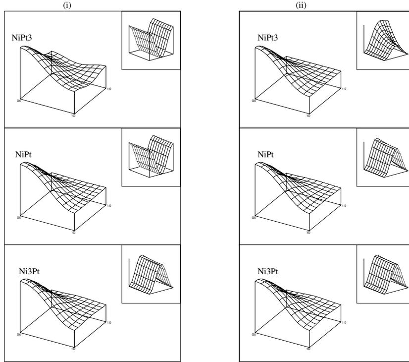
**Figure 5.** The  $V(\vec{k})$  surface for NiPt alloy systems with potential parameters calculated with the choice of (i) charged spheres and (ii) charge neutral spheres on the  $k_z = 0$  plane. The figures in the inset are the corresponding rescaled  $V(\vec{k})$  surfaces on the  $k_z = 0$  plane along the (100) to (110) direction to view the minima.
