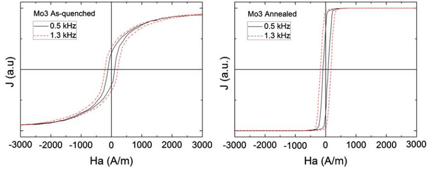
**Fig. 2.** Hysteresis loops at a frequency of 0.5 kHz (black solid line) and 1.3 kHz (red dashed line) of  $\text{Fe}_{73.5}\text{Si}_{13.5}\text{Nb}_{3-x}\text{Mo}_x\text{B}_9\text{Cu}_1$  ( $x=3$ ). Left: as-quenched ribbon. Right: annealed ribbon. (For interpretation of the references to color in this figure legend, the reader is referred to the web version of this article.)
