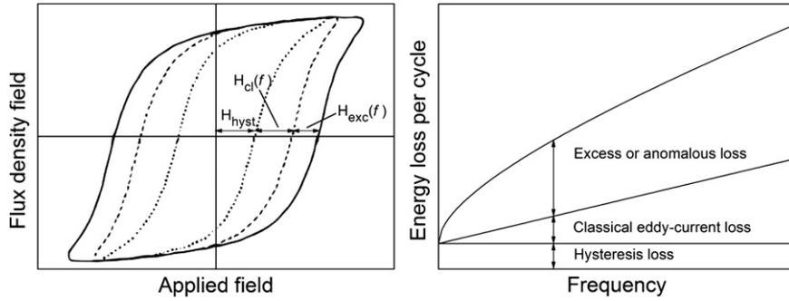
**Fig. 1.** Left: contributions to the coercivity in the hysteresis loop—static hysteresis, classical eddy currents and anomalous or excess field (modified from Ref.[3]). Right: contributions to the energy loss per cycle as a function of the frequency of the magnetizing field.
