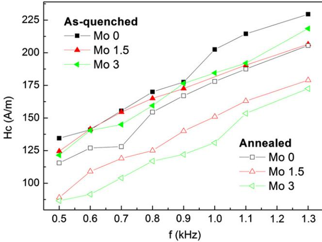
**Fig. 3.** Coercivity as a function of the frequency of the applied field for as-quenched (solid symbols) and annealed (empty symbols) samples. Lines between experimental points are drawn as guides for the eyes.
