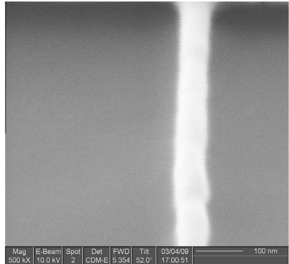
Fig. 3. SEM image showing 60 nm wire with undulating instability.
