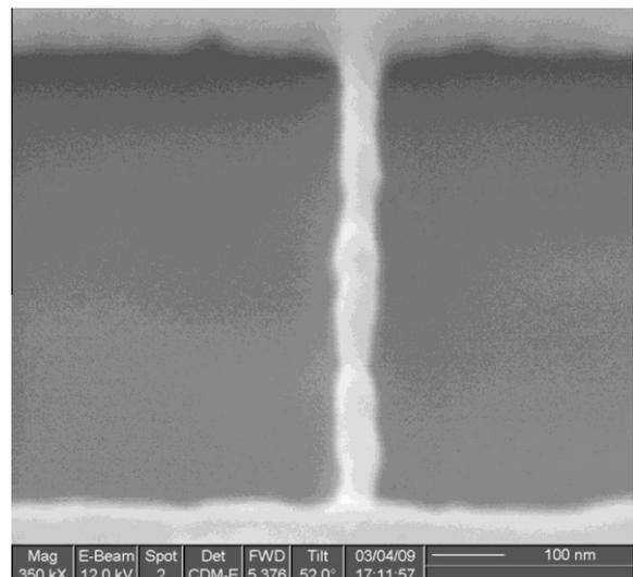
Fig. 4. SEM image of the nanowire below 50 nm in diameter with periodic undulation of the width.
