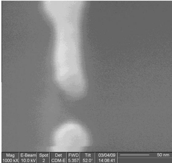
Fig. 6. SEM Image showing fragmented nanowire.
