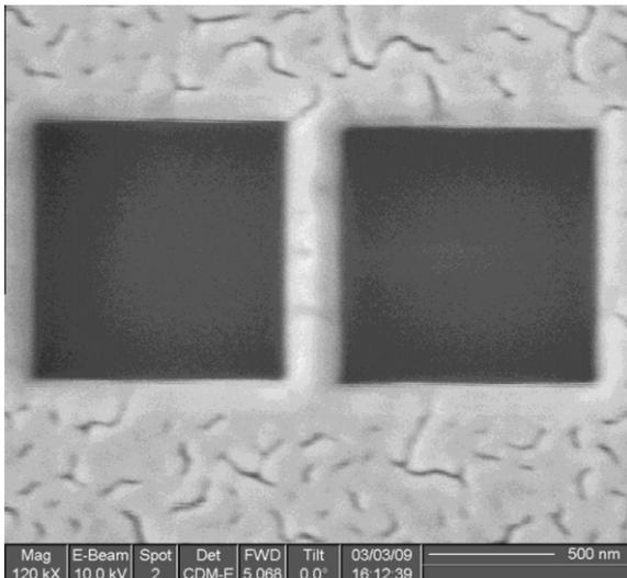
Fig. 2. SEM image of the 200 nm gold wire showing stable morphology.
