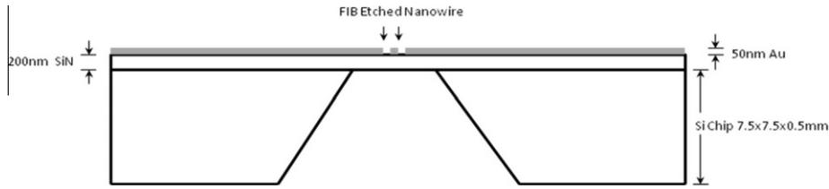
Fig. 1. Cross-section of the  $\text{Si}_3\text{N}_4$  membrane with FIB etched nanowire.
