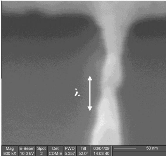
Fig. 5. SEM image showing onset of droplet formation in the unstable nanowire.
