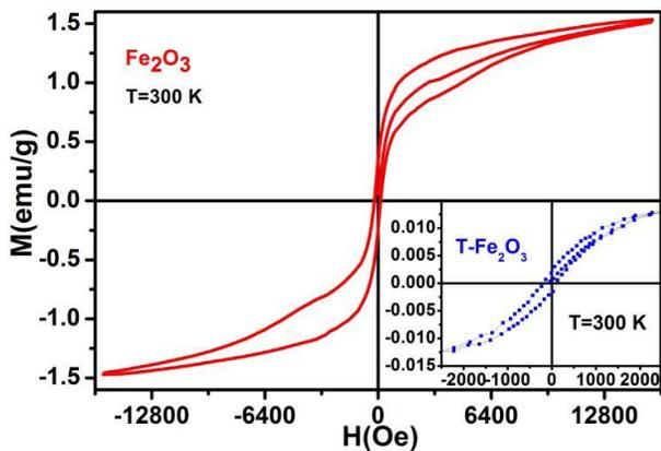
Fig. 2. Magnetization versus applied magnetic field plot for the as-prepared bare  $\alpha$ - $\text{Fe}_2\text{O}_3$  NPs. In the inset hysteresis loop of T- $\text{Fe}_2\text{O}_3$  NPs indicates ferromagnetic nature.
