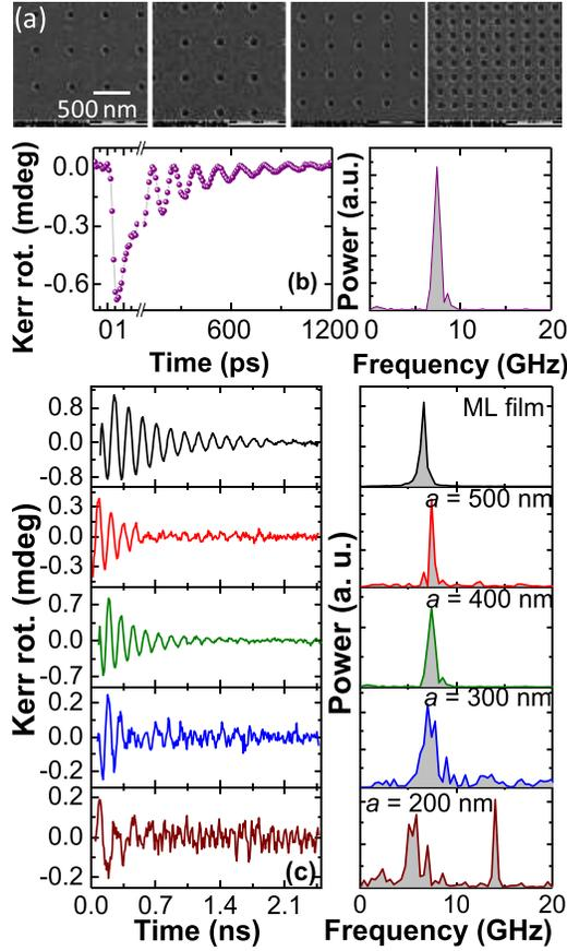
FIG. 1. (a) Scanning electron micrographs of the antidot lattices (ADLs) with lattice constant  $a$  varying as 500, 400, 300, and 200 nm. (b) Typical TR-MOKE signal and corresponding spin wave spectrum for ADL with  $a = 400$  nm. (c) Areal density dependence of the TR-MOKE signal with the bi-exponential background subtracted and the spin wave spectra of the ADLs and a ML film at  $\mu_0 H = 0.084$  T.
